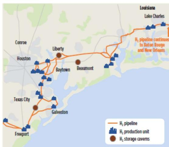
**FIG. 4.** Existing H<sub>2</sub> system in the U.S. Gulf Coast region. Sources: H2Tools, USDOT-PHMSA, Air Liquide, Air Products, Praxair.
